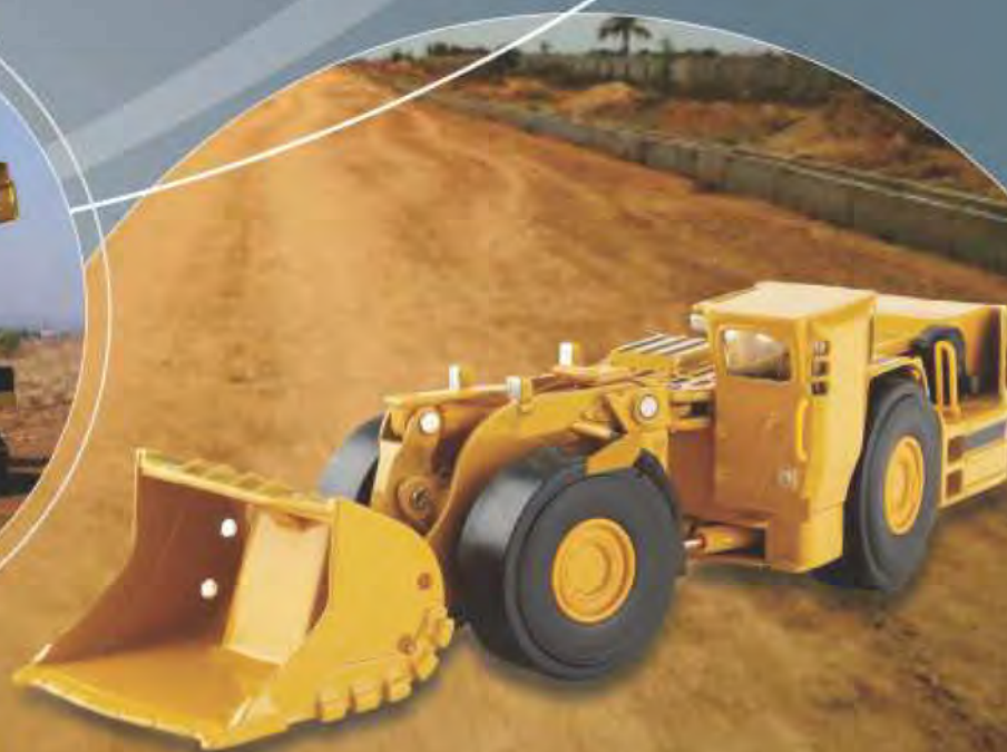
A LOAD-HAUL-DUMPER, POWERED BY A KIRLOSKAR ENGINE
